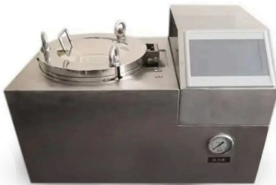
Deprotection Equipment for Cutting DNA Sequence
