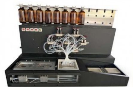
HY 192 DNA RNA Oligo Synthesizer for High Throughput
